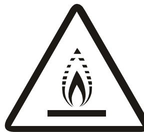
Warning: low burning velocity material (For products containing R32 refrigerant comply with the IEC 60335-2-40:2018 standard only)
